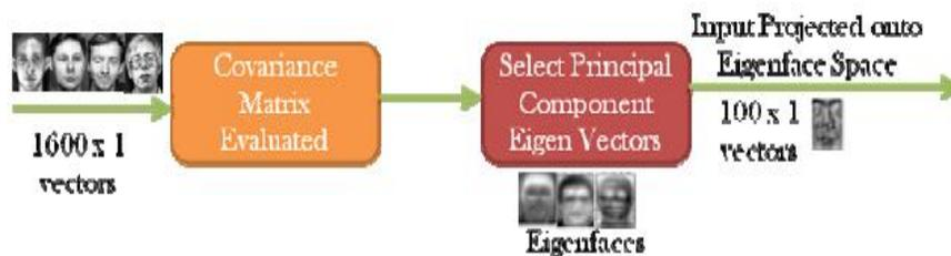
Fig.2 Flowchart for Dimensionality Reduction step
