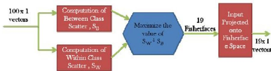
Fig. 3. Flowchart for Feature Extraction using LDA
