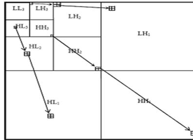
**Fig.1. 3-level multi wavelet transforms**
