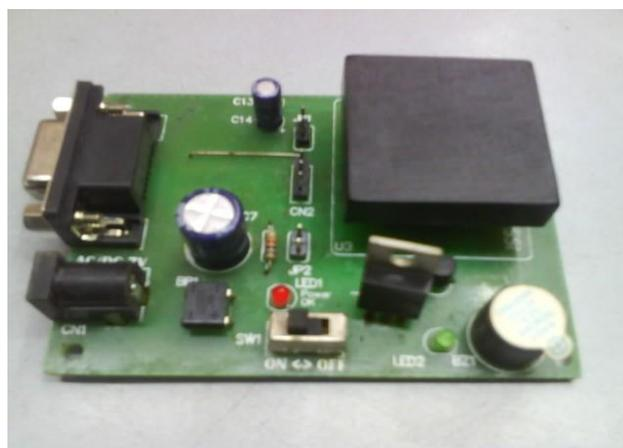
Fig.2.2 RFID Reader Board
