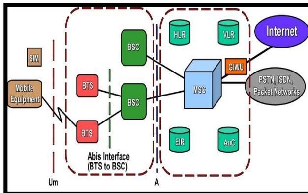
Fig.2.1 GSM Architecture
