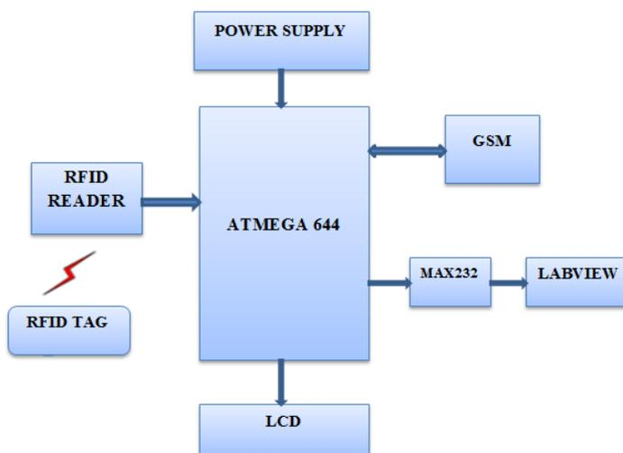
Fig.1.2 Block Diagram of School module.
