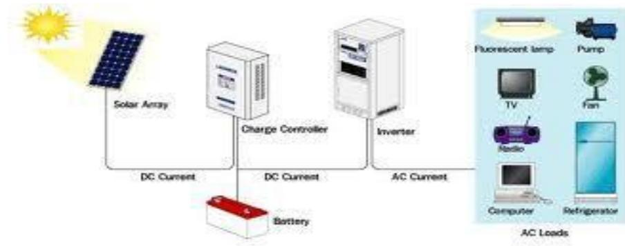
Figure 2: Functional View of standalone Solar system
