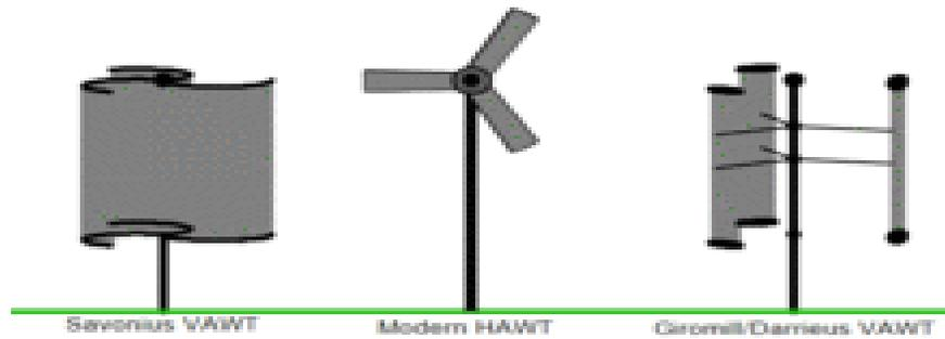
Figure 3: Types of wind turbines (Savonius VAWT, Modern HAWT & GDarrieus VAWT)
