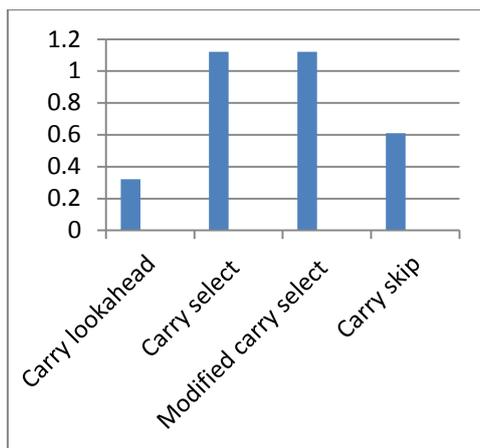
Fig.7 Propagation delay
