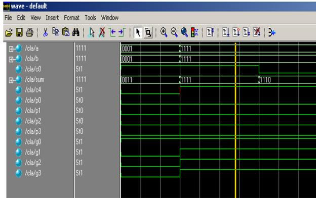
Fig.3 Modified carry select adder
