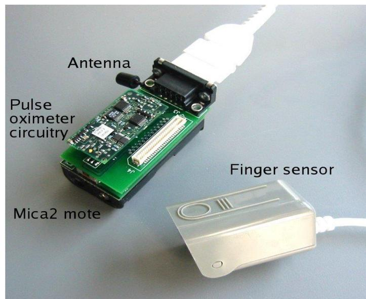
Fig. 2 Mote Based Pulse Oximeter
