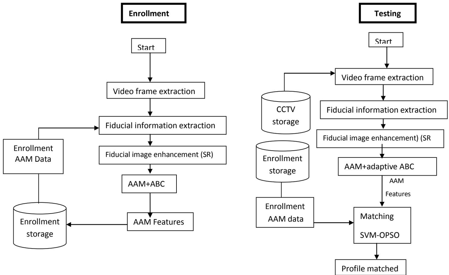
Figure 1. The proposed 2.5D Face Recognition Technique
