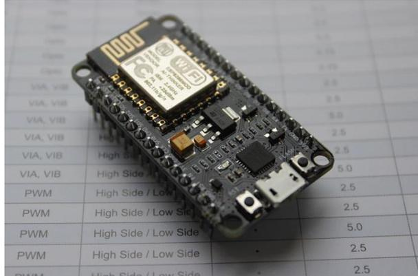
**Fig 3: Representation of the NodeMCU (ESP8266)**
