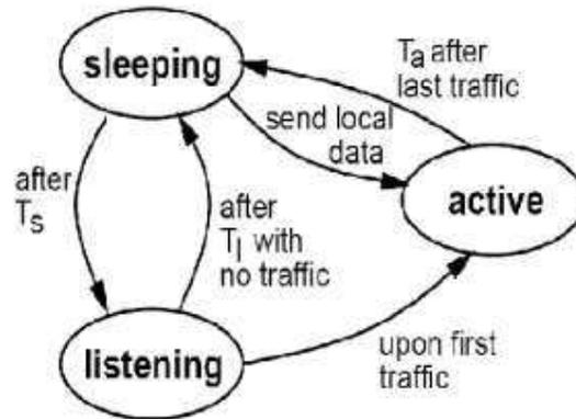
when no messages are being processed i.e., when the node is in not active, An inactive node listens for activity for  $T_l$  seconds, and if no activity is seen during that period of time it sleeps for  $T_s$  seconds before listening again.
