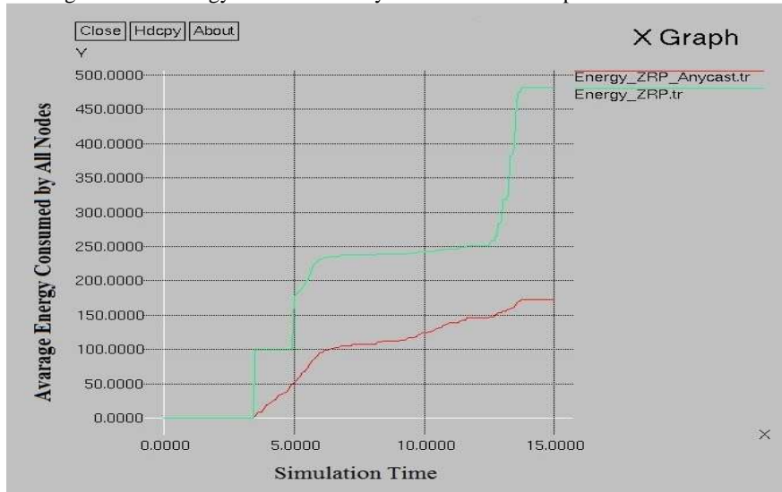
Figure 6.1 Graph between average energy consumed by all nodes and simulation time
