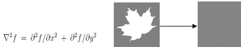
Fig 5 Initial image and Laplacian image
