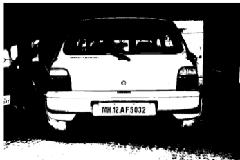
Fig.3: Output of Otsu's algorithm
