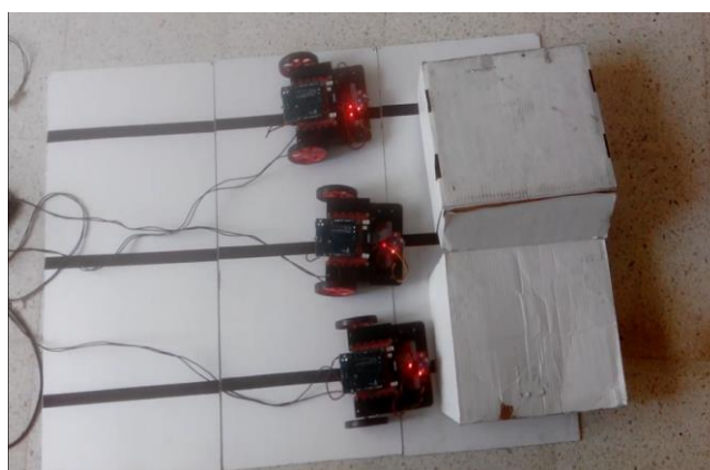
Fig. 9 Three robots pushing the box
