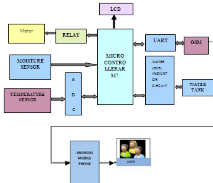
Fig.3: Block Diagram of the Irrigation Control System
