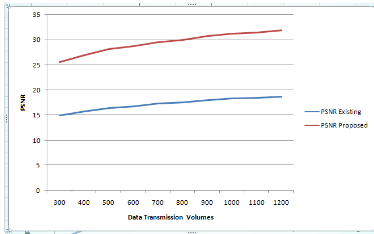
Figure 2: Graph of PSNR values collected from the UWSN simulation model
