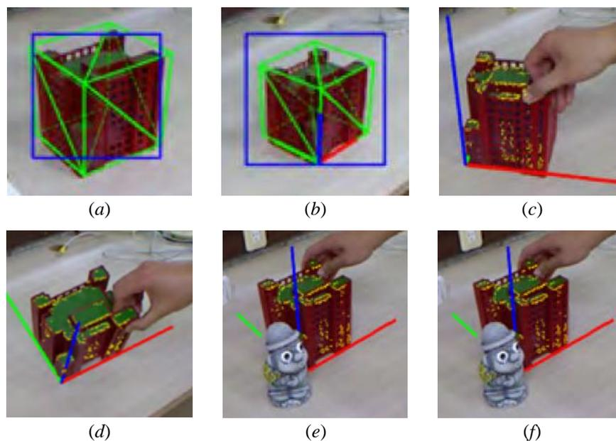
Fig. 8 Real-time 3D object detection and tracking: (a) object selection, (b) DOT template of the object and the corresponding depth map from the new viewpoint, (c) tracking 3D object under viewpoint 1, (d) tracking 3D object under viewpoint 2, (e) 3D object under partial occlusion, and (f) 3D object under fast motion [40].
