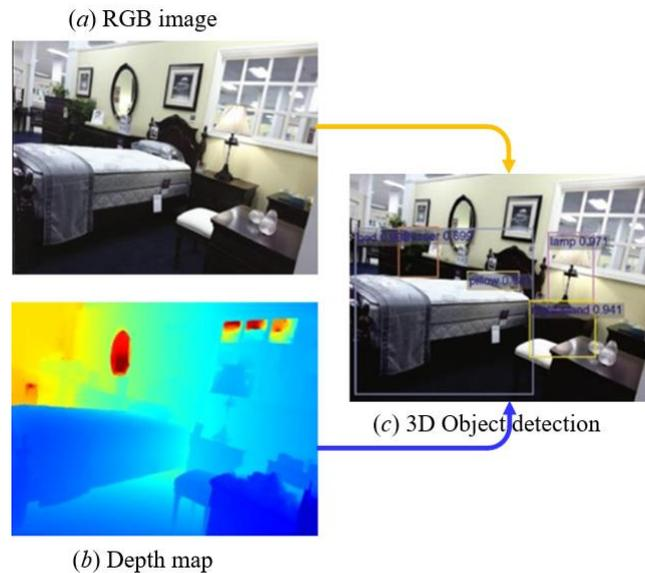
Fig. 7 RGB-D Feature map: (a) RGB image, (b) depth map, (c) 3D object detection [39].
