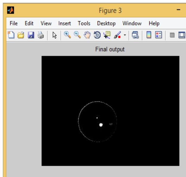
Fig 4: Output of Circular Hough Transformation
