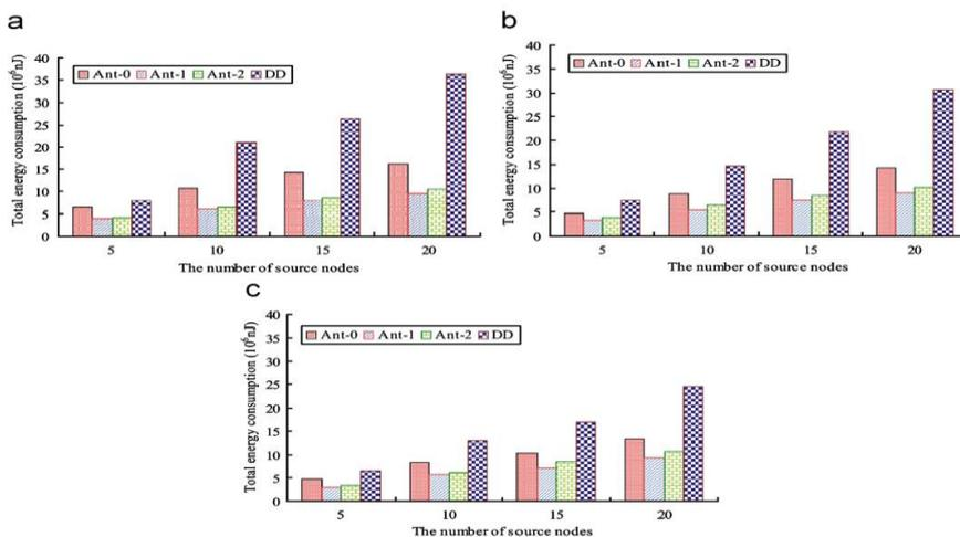
Fig 2: Total energy consumption vs. the number of source nodes for methods Ant-0, Ant-1, Ant-2, and DD: (a) R = 10, (b) R = 12, (c) R=14.
