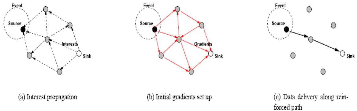
Figure 1: A simplified schematic for directed diffusion.
