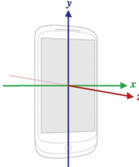
Fig. 2 Orientation of the Android device axes
