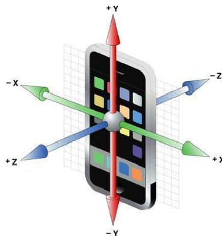
Fig. 1 Orientation of the iPhone device axes
