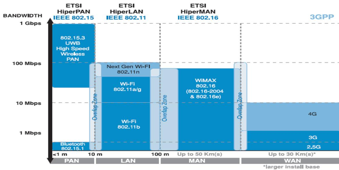
Fig 1. Bandwidth and coverage of wireless technologies [2]
