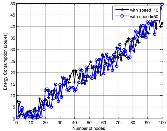
Fig.6 Energy Consumption vs. no. of nodes for speed 10m/sec and 50m/sec
