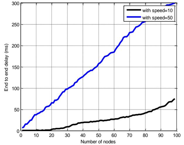
Fig.4 end to end delay vs. no. of nodes for speed 10m/sec and 50m/sec
