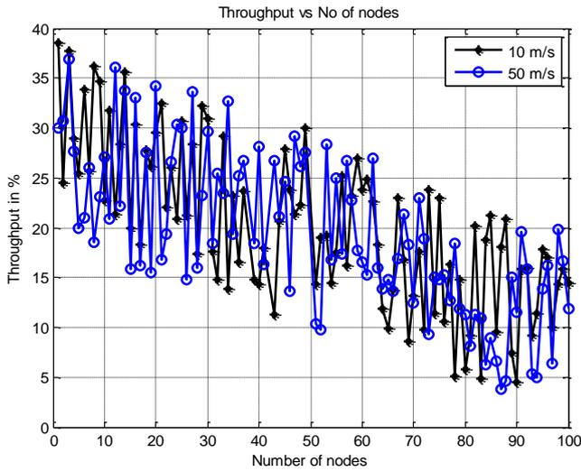
Fig.3 Throughput vs. no. of nodes for speed 10m/sec and 50m/sec
