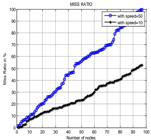
Fig.2 Packet miss ratio vs. no. of nodes for speed 10m/sec and 50m/s
