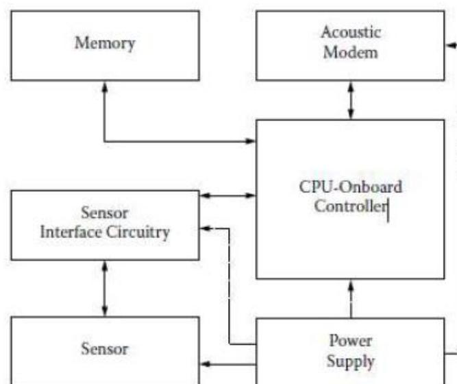
Fig 2: Underwater Sensors
