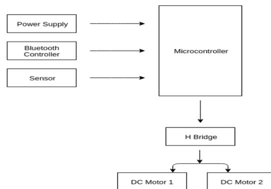
Fig. 3.1 Block Diagram of voice controlled wheelchair
