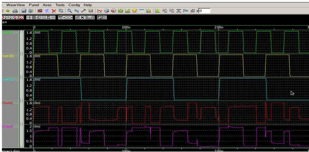
Fig 6: Output Waveform of Conventional 10T Full Adder
