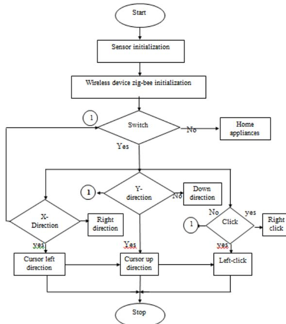
Fig. 4. Flow chart of hand gestured mouse control.
