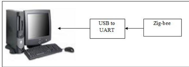
Fig.2 Block diagram of Computer Application Interface section of human mouse
