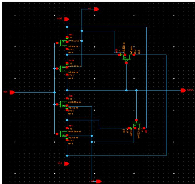
Fig 3. Schematic of VTCMOS Schmitt Trigger
