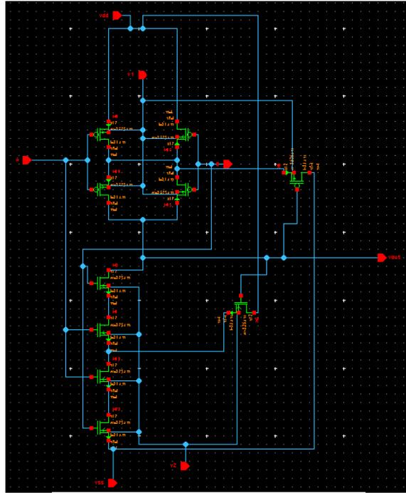
Fig 5. Schmitt Trigger NAND gate using VTCMOS
