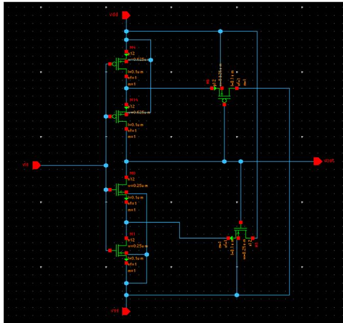
Fig 2. Schematic of basic CMOS Schmitt Trigger
