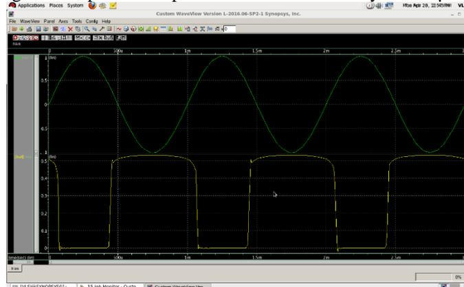
Fig 7. Output waveform of VTCMOS Schmitt Trigger
