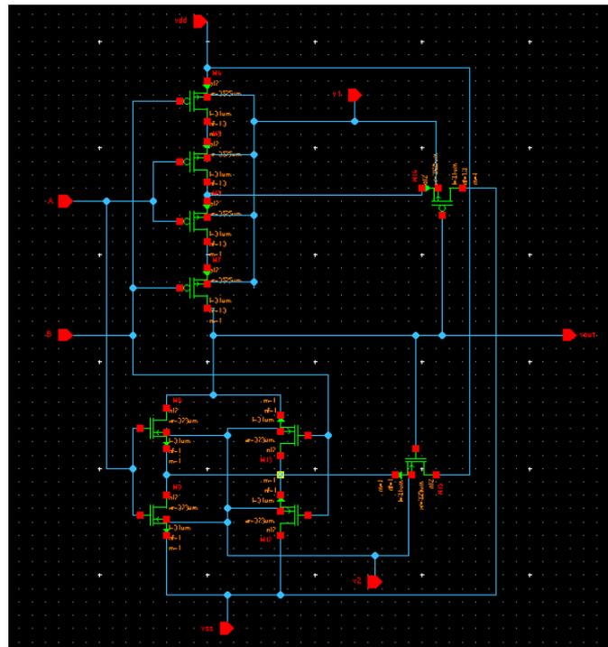
Fig 4. Schmitt Trigger NOR gate using VT MOS
