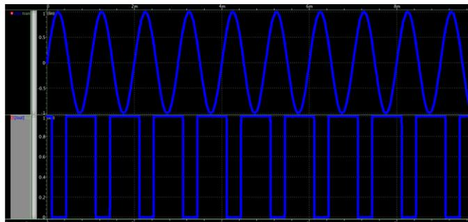
Fig 6. Output waveform of Basic Schmitt trigger
