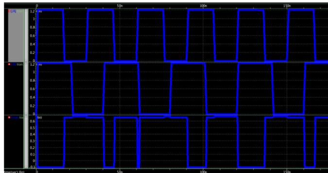
Fig 9. Output waveform of Schmitt Trigger NAND gate using VTCMOS
