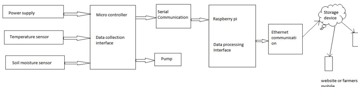
Fig 1.connection of sensor to raspberry pi
