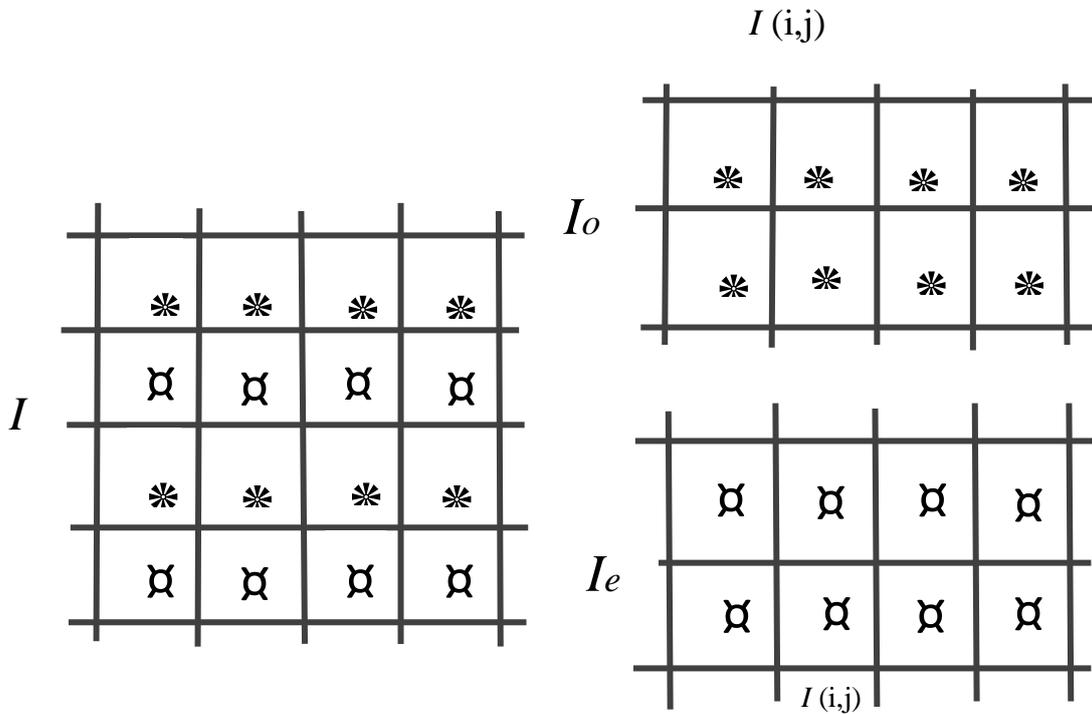
**Fig.(2): Input image that decomposed into even and odd sub-images [20].**
