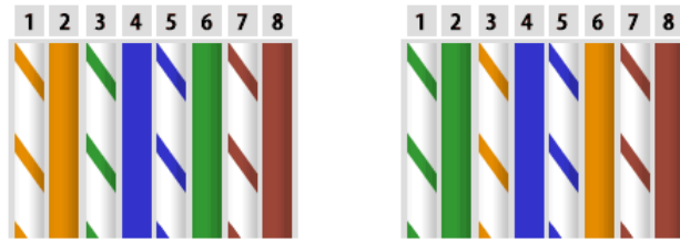
Fig. 2 Crossover Cable Design
