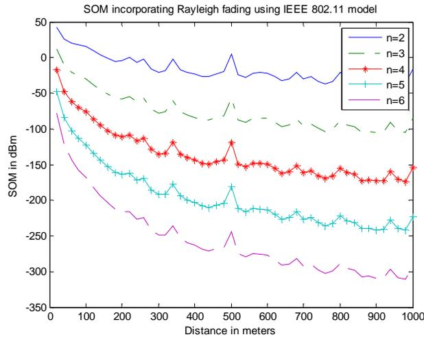
Figure 4. SOM Estimation under Rayleigh fading for VANET
