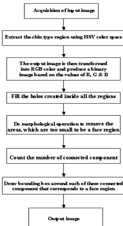
**Figure 4. Flow diagram of the proposed algorithm**
