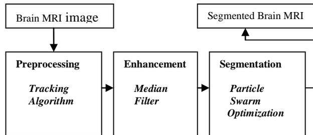
Fig1. Block diagram for proposed system.
