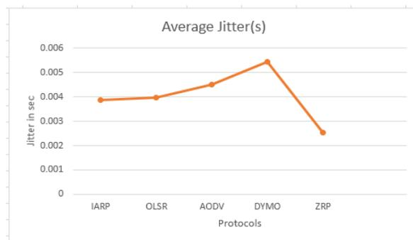
Fig.4. Average Jitter in Seconds
