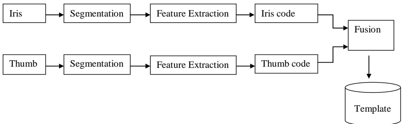
Fig. 2: Proposed Multibiometric System
