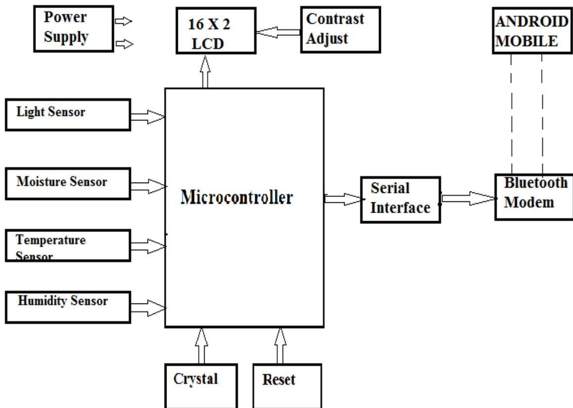
Figure 1: Block diagram of Android based Greenhouse Maintenance and Controlled System
