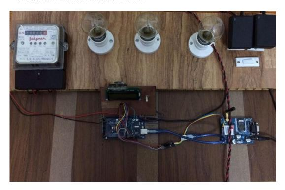
• The units consumed by the customer is continuously displayed on the LCD screen with the appropriate cost of that units:
