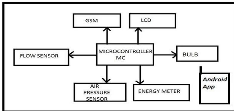
Fig 7: Representation of metering system
