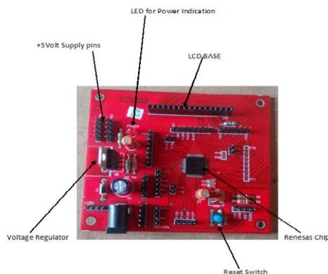
Fig 6: 64 pin Renesas Microcontroller board
