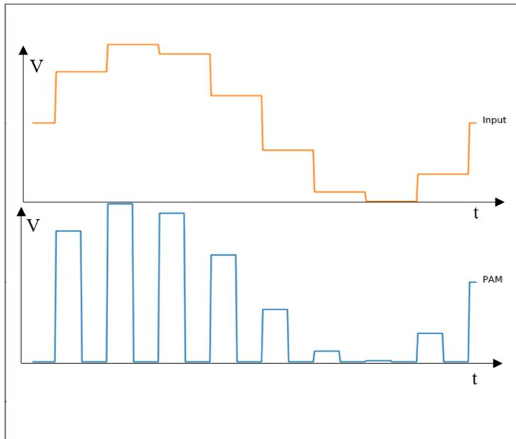
Figure 2.1: Input and output of a sample PAM.
