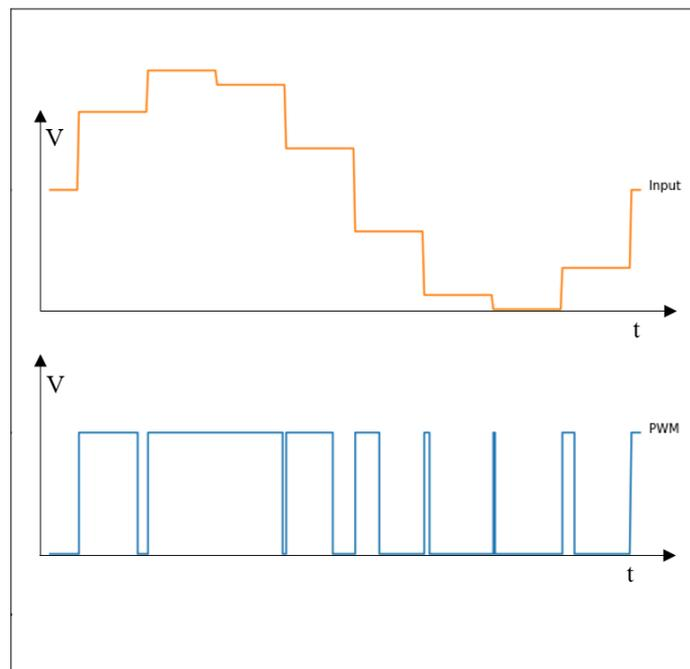
Figure 2.2: Input and output of a sample PWM.
