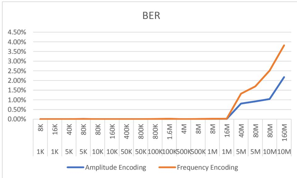
Figure 4.2: BER versus bandwidth for the proposed hybrid method using amplitude and frequency encoding.
