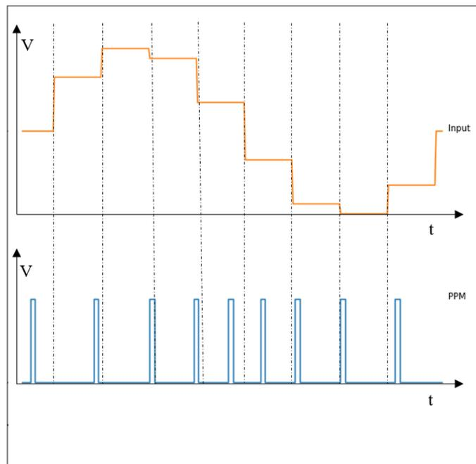
Figure 2.3: Input and output of a sample PPM.
