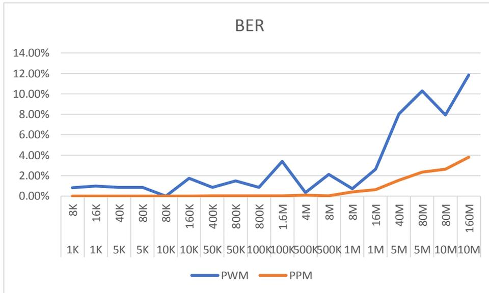
Figure 4.1: BER versus the pulse rate and bandwidth of the PWM and PPM modulations.
