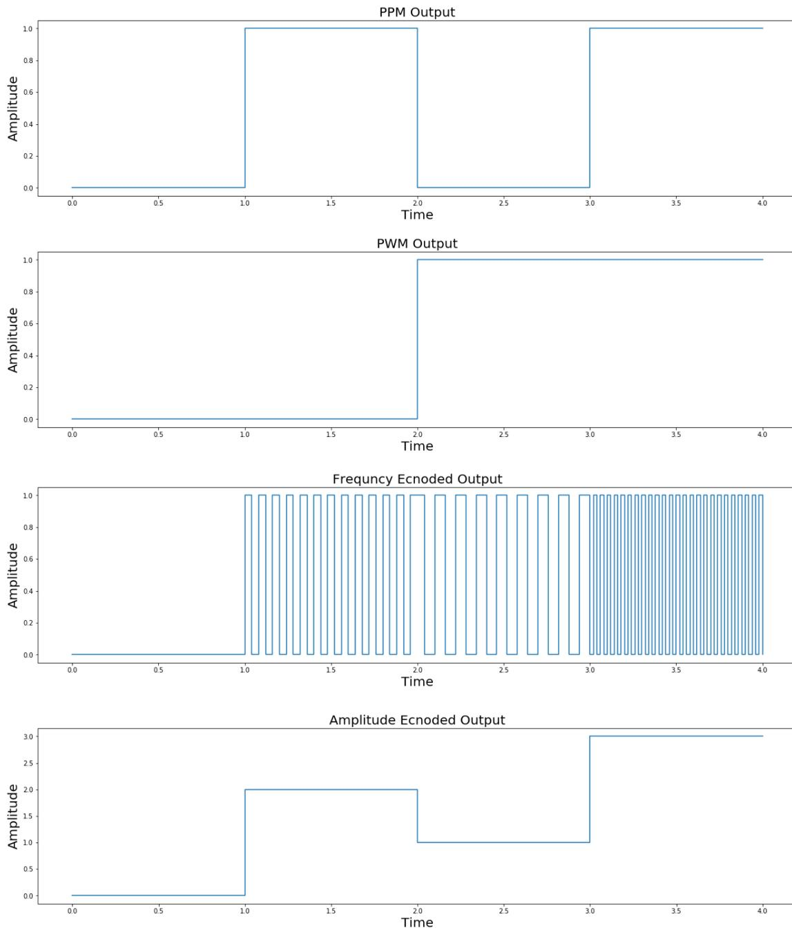
Figure 3.2: Outputs of the frequency and amplitude encoding techniques.
