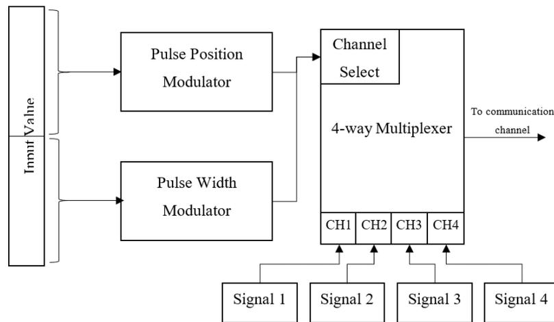
Figure 3.1: Encoding the output of the modulators in the proposed hybrid method.
