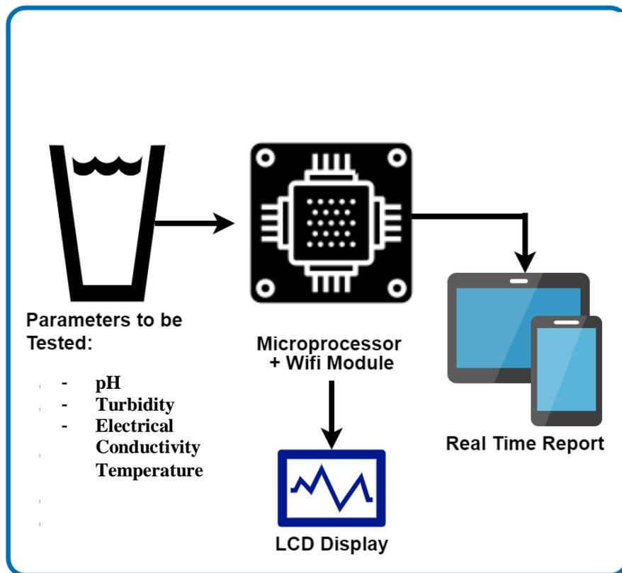
**Figure 7.** Data Flow Diagram of the Water Quality Monitoring System
