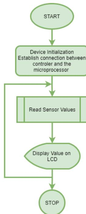
**Figure 3.** Flow Chart for Water Quality Monitoring System
