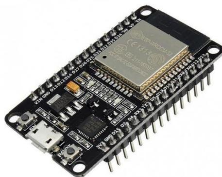
**Figure 2.** The ESP32 module to communicate with Arduino Board.
