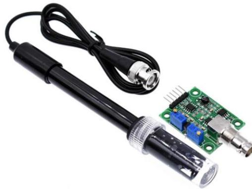
**Figure 3.** The pH-4502c sensor.
