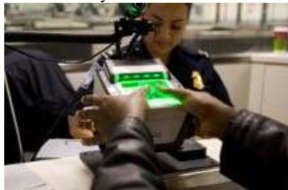
Fig 11 Fingerprint reader used for border control by the US department of Homeland Security
