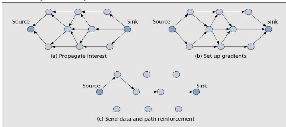
Fig 5: Interest diffusion in wireless sensor network [4]
