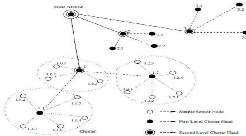
Fig 5: Hierarchical Routing
