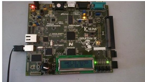
Fig.10 FPGA Implementation results of UART with BIST Architecture
