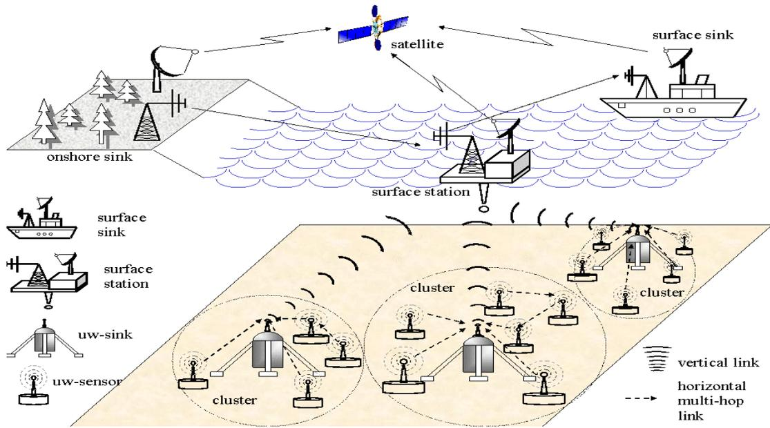
**Fig2. Architecture of 2D underwater sensor networks REF- Georgia Institute of Technology**
