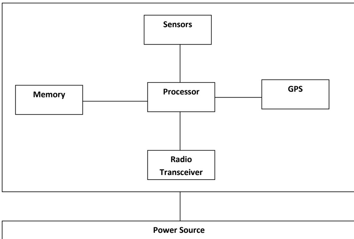
**Fig1. Components of WSN Node**
