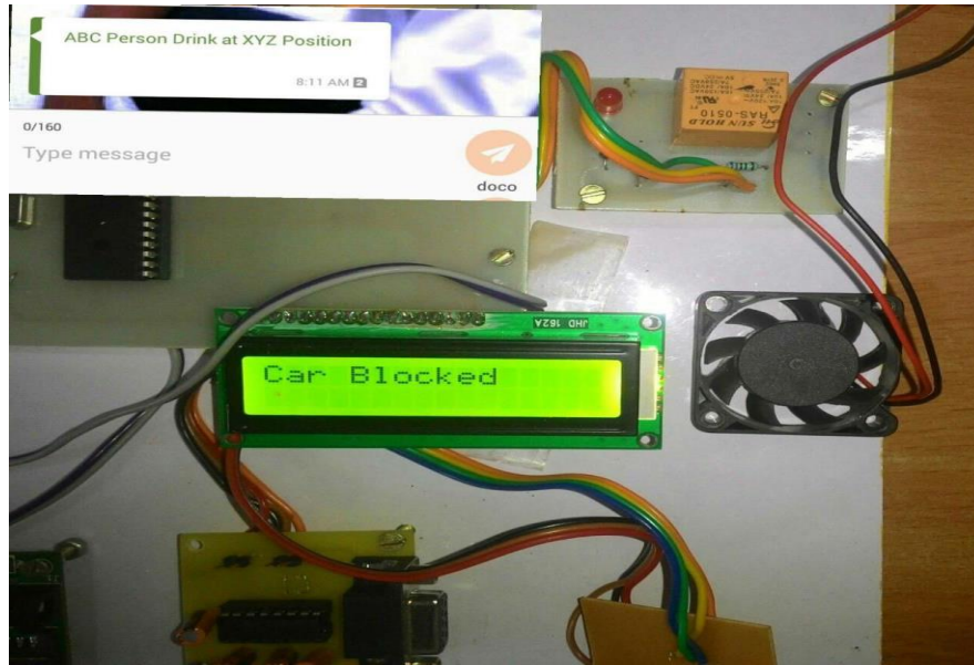
Figure 8. Car get blocked as alcohol sensor detects alcohol in car.
