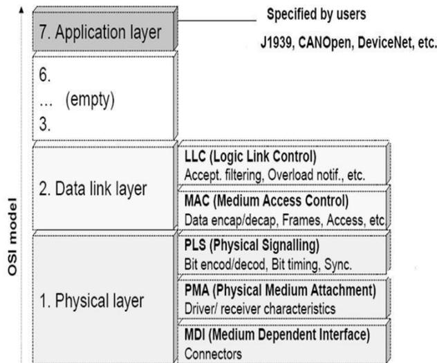
Figure 2. Hierarchical structure of CAN BUS
