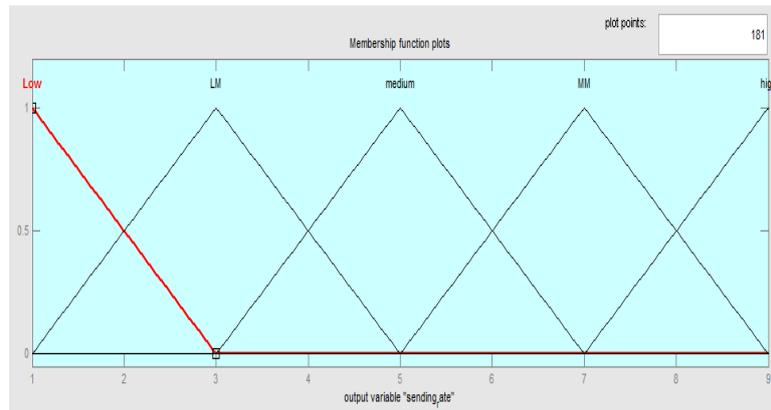
Fig. 4 Membership function used for output variable
