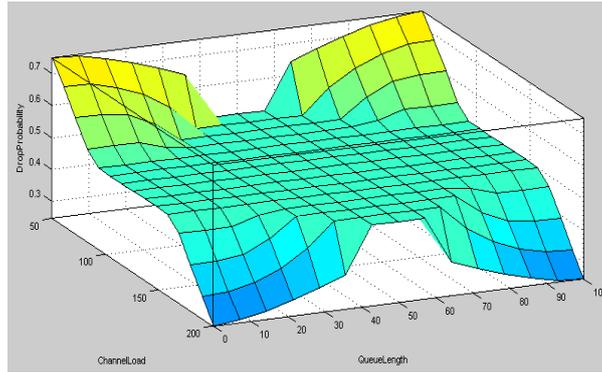
Fig. 14 Surface view showing channel load, queue length and Drop probability
