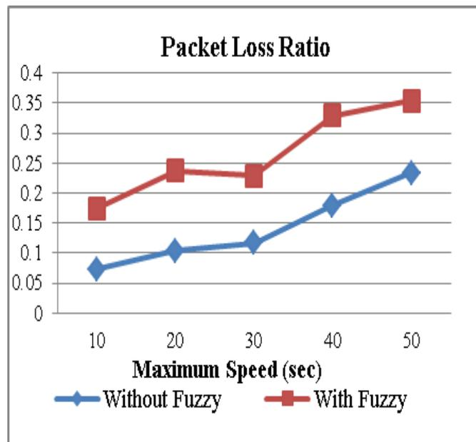
Fig.8 Packet loss ratio with varying maximum speed
