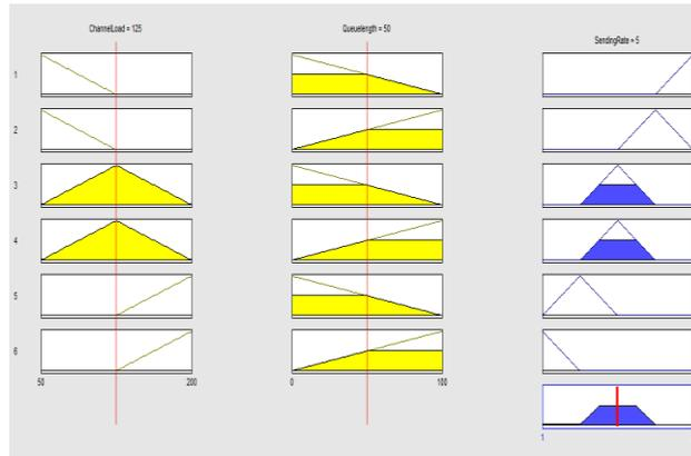
Fig. 5 Rule view for Channel load, Queue length and Sending rate
