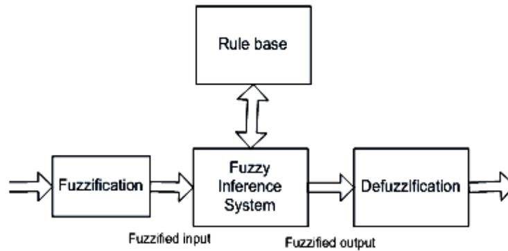
Fig.1 Block diagram of fuzzy logic controller system
