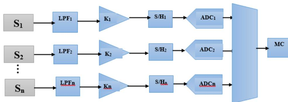
Fig3. 2. Structures of the Data loggers with Multi-ADC
