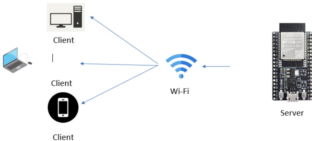
Figure 5. sending data over Wi-Fi channel
