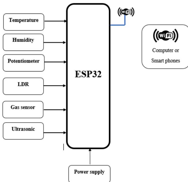
Figure 3. The block diagram of the data logger based on ESP32
