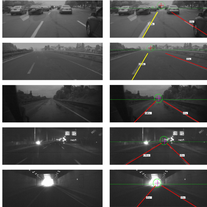
Fig.5 (a) Urban road and Vehicle disturbing (b) Worn off marks (c) Rainy (d) Night (e) Exit of a tunnel Original image tracking results
