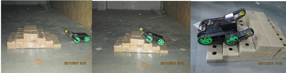
Fig.5 Different poses of the surveillance robot while climbing staircase
