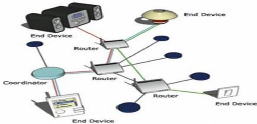
**Figure 2 Generalized ZigBee Network[6]**
