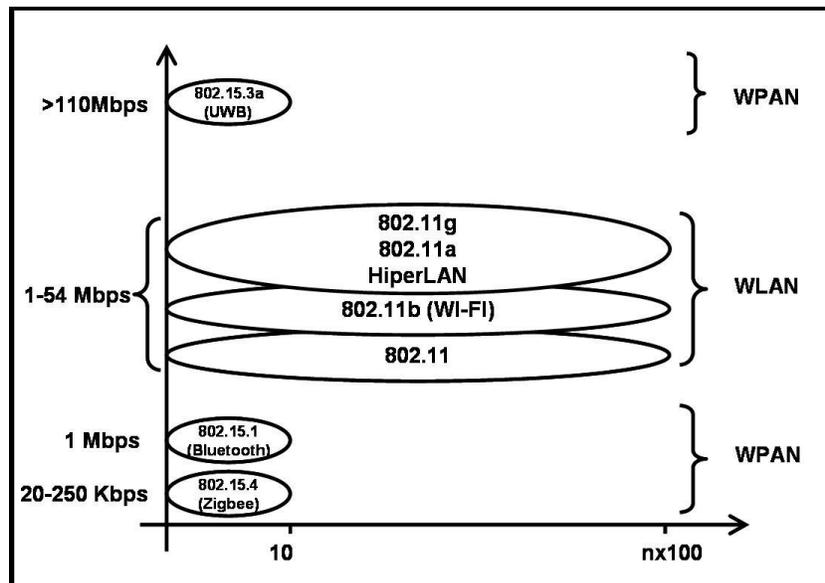
Figure 1 showing WPAN, WLAN, WPAN(Zigbee)
