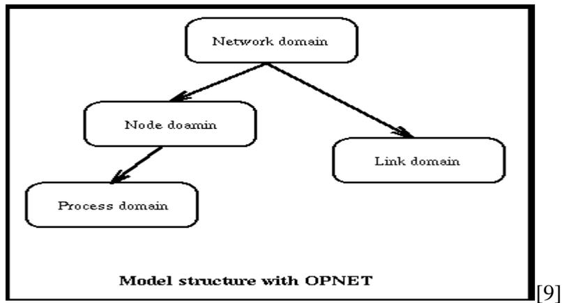
**Figure 3 Model structure with Opnet**
