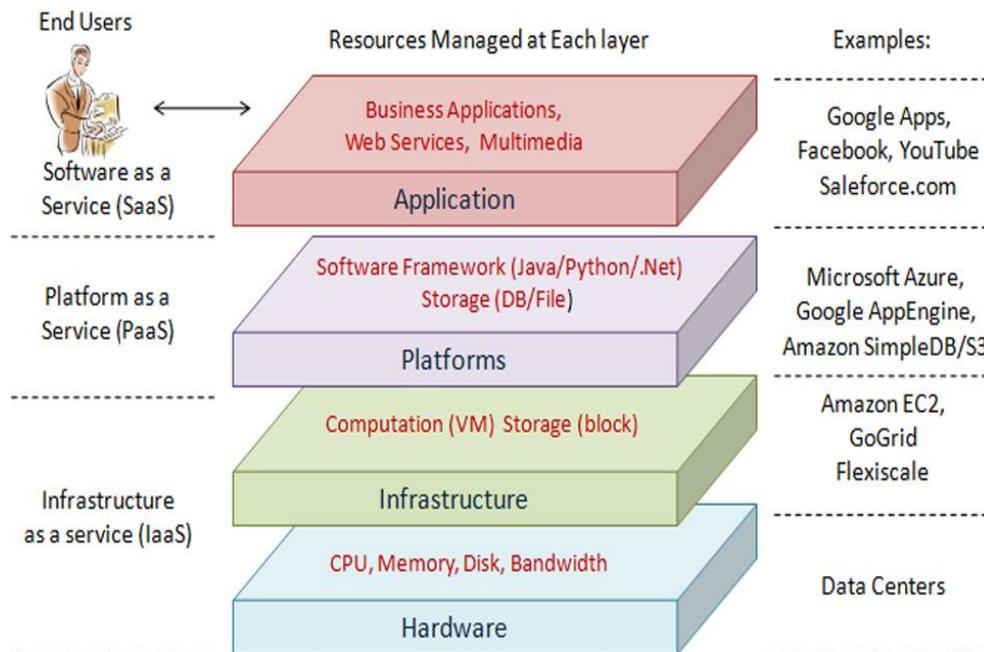
Figure 3 Cloud Computing Architecture [1]
